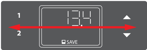
Fig. 51. The LegaDrive Touch Inlay handset lock is activated and deactivated by swiping to the left or right
