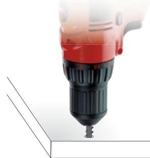
3 - Screw the assembly fitting into the face bored panel using a cross screwdriver.
